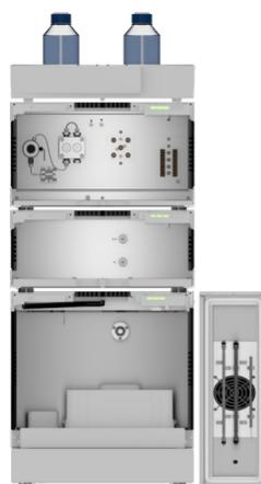
**Fig. 8** SEC system setup; from top to bottom: eluent tray with bottles, pump, refractive index detector (RID), autosampler; right: thermostat with columns.
