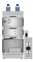
**Fig. 7** GPC system setup; from top to bottom: eluent tray with bottles, pump, refractive index detector (RID), autosampler; right from top to bottom: degasser, thermostat with column.
