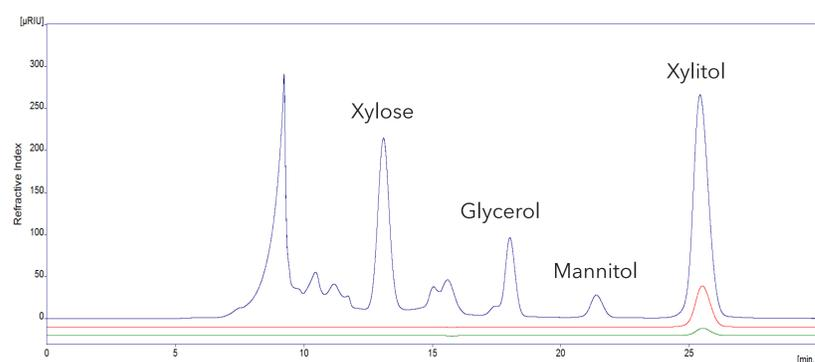
**Fig. 2** Overlay of analytical chromatograms; blue - fermentation mash (1:2 dilution); red - fractionation sample from Fig. 1; green - xylitol standard 1 mg/mL; 10 µl each; EK Ca 300 × 8 mm; 75 °C
