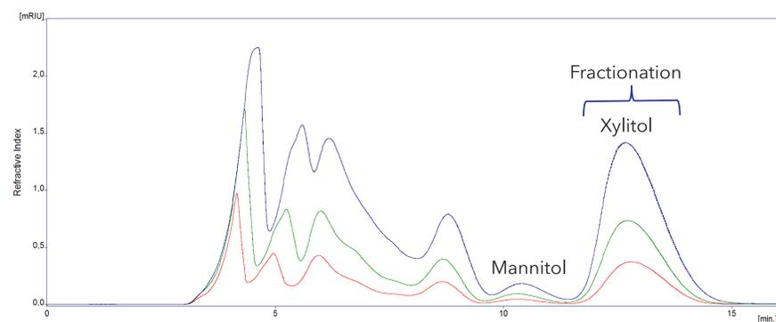
**Fig. 1** Chromatogram overlay of different injection volumes from fermentation mash (1:2 dilution); red - 0.5 mL, green - 1 mL, blue - 2 mL; blue brackets - fractionation area 2 mL injection; EK Ca 150 × 20 mm; 4 mL/min; 60 °C
