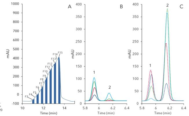
**Fig. 3** Fraction analysis of preparative online-SPE purification (Fig.2) of rebaudioside A (1) and stevioside (2); A) fractionation of target peak, 5 mL fractions B) F3 (blue), F4 (red), F5 (green), F6 (light blue); C) F7 (red dashed), F10 (blue dashed), F12 (green dashed), F15 (light blue dashed)
