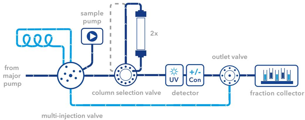
Fig. 6 Flow scheme for the sample pump set up for two step purification.
