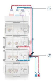
**Fig.2** System setup with the old (1) and new (2) sampling point. The sample extract is shown in red, the sample raffinate in blue.
