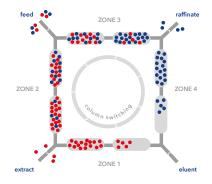
Fig. 1 Operation mode of the SMB.
