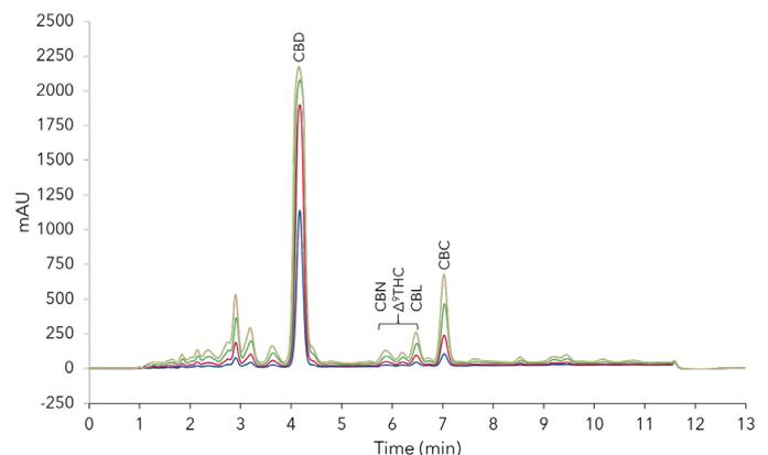
**Fig. 6** Volume overload study with methanol method on C18 10  $\mu$ m particle. 2  $\mu$ l, 5  $\mu$ l, 10  $\mu$ l, 15  $\mu$ l injection of 50 mg/ml CBD-Loges sample; C18, 10  $\mu$ m, 150 x 4.6 mm ID.
