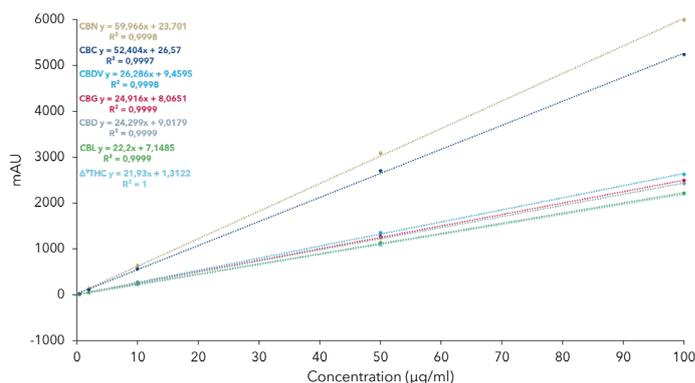
**Fig. 3** Calibration curves and linearity for the cannabinoids CBDV, CBG, CBD, CBN, Δ<sup>9</sup>-THC and CBL for analytical ACN method at 228 nm.
