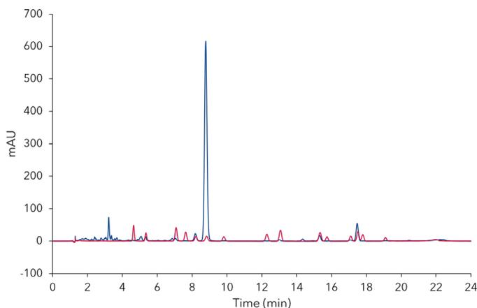
**Fig. 1** Overlay chromatograms of CBD oil sample (blue) and mixture of 16 Cannabinoids (red). CBD oil sample 5 mg/ml; standard concentration 5 µg/ml each; 10 µl injection, 228 nm; C18P, 3 µm, 150 x 4.6 mm ID.
