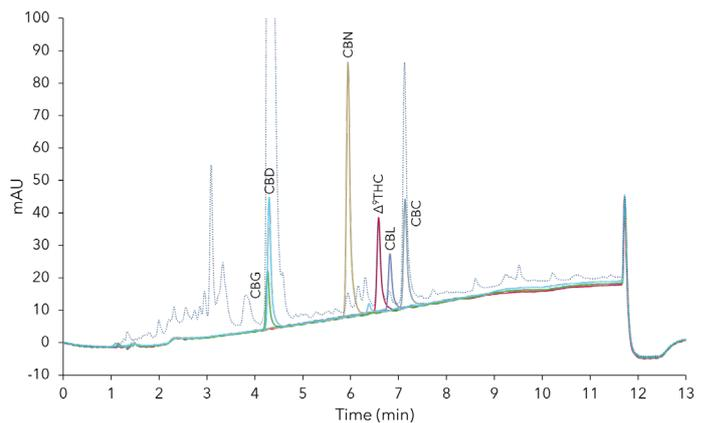
**Fig. 5** Detailed view overlay of CBD oil sample and single standard chromatograms. CBD-Loges oil (dashed line), standards in elution order: CBG (5  $\mu$ g/ml), CBD (10  $\mu$ g/ml), CBN (10  $\mu$ g/ml),  $\Delta^9$ -THC (10  $\mu$ g/ml), CBL (5  $\mu$ g/ml), CBC (5 $\mu$ g/ml), C18, 3  $\mu$ m, 150 x 4.6 mm ID.
