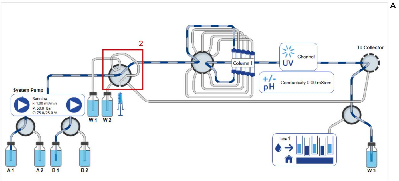
After the sample injection and an isocratic washing step, the elution starts after 5 ml with beginning of the gradient (Fig. 6 B.1). At this time point the multi-injection valve should be switched back to the manual load position (Fig. 6 A+B.2).
