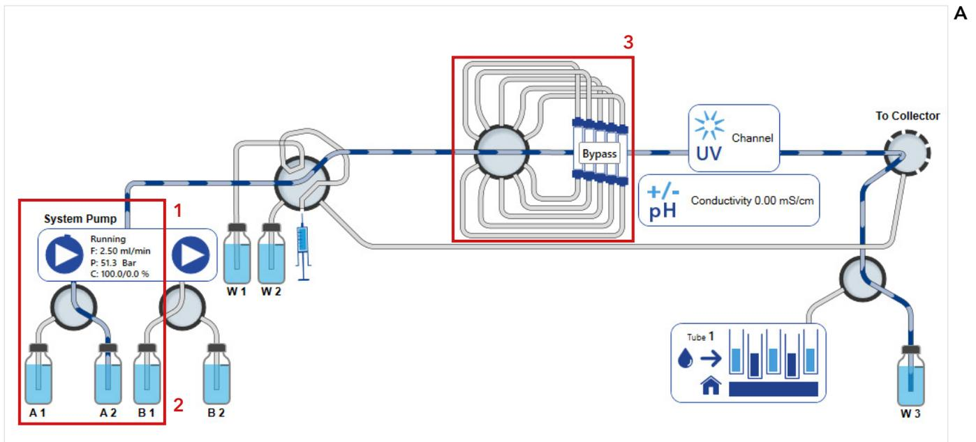
the UV detector and the multi-injection valve for “Peak storage stop”. At the end of the run purified protein is stored in the injection loop and can be further purified via the second column in the next step without manual interference.
