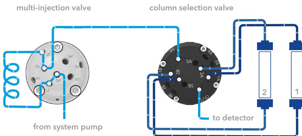
Fig. 3 Connection of the column selection valve.
