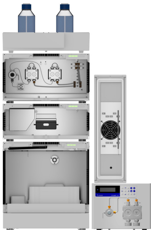
Fig. 3 KNAUER UHPLC system with additional preparative pump, used for the experiments
