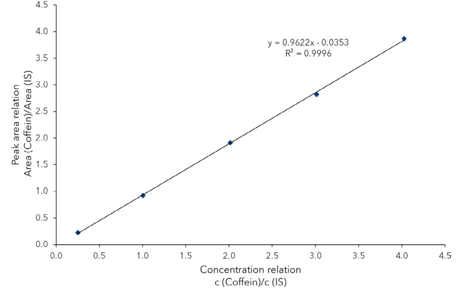
Fig. 1 Calculated ISTD calibration curve of caffeine (Mobile Control)
