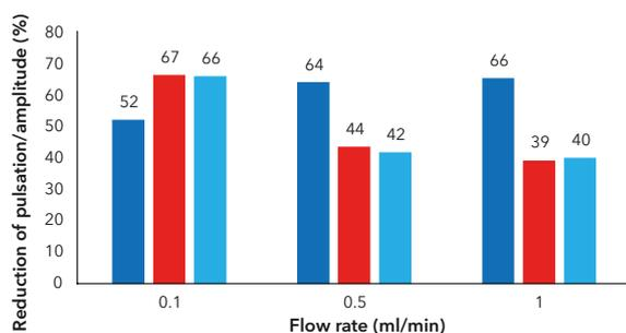
**Fig. 1** Comparison of the relative reduction of the pulsation for different flow rates and different back pressure (dark blue) ~1.5 bar; (red) ~4.5 bar (light blue) ~10 bar with water
