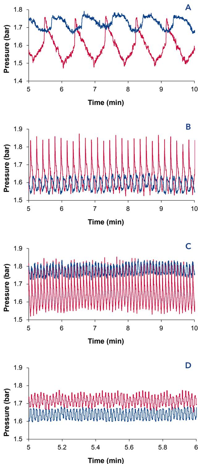
**Fig. 2** Overlay of the external pressure signal at different flowrates, approx. 1.5 bar back pressure and water as eluent. Pressure signal without pulse damper (red), pressure signal with pulse damper (blue); (A) 0.1 ml/min; (B) 0.5 ml/min; (C) 1ml/min; (D) 5 ml/min
