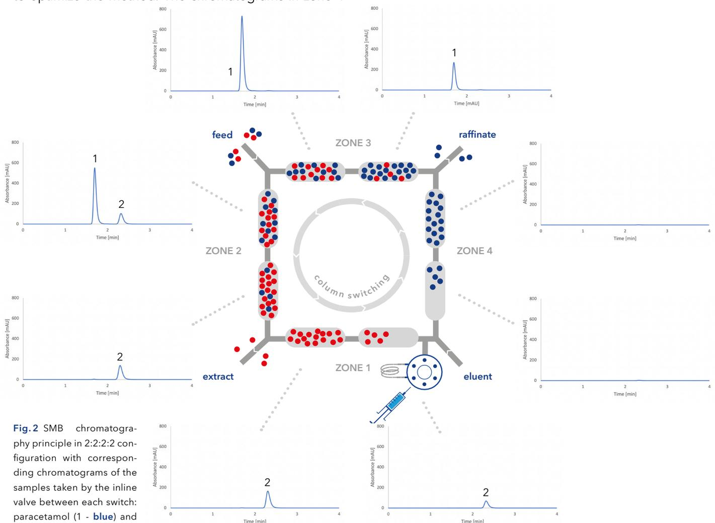
**Fig. 2** SMB chromatography principle in 2:2:2:2 configuration with corresponding chromatograms of the samples taken by the inline valve between each switch: paracetamol (1 - blue) and caffeine (2 - red).
