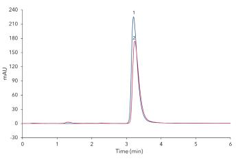
**Fig. 4** 1 - Step 4 Automated analysis, 10  $\mu$ l injection, 1 ml/min flow, caffeine area: 2807,6 mAU·s. 2 - Step 5 Manual analysis of the fraction from Fig. 2, 10  $\mu$ l injection, 1 ml/min flow, caffeine area: 2283,6 mAU·s.
