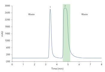
**Fig.3** Step 1 Purification with fractionation window (green), 50 μl injection, 15 ml/min flow. 1 - Paracetamol, 10 mg/ml; 2 - Caffeine, 15 mg/ml.
