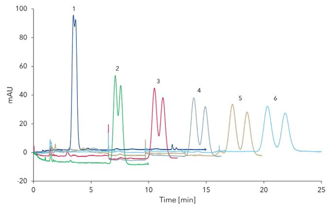
**Fig. 4** Overlay of chromatograms for alternate pumping recycling chromatography. Comparison of six measurements with increasing cycle numbers (1 to 6); 3.5 mL/min; 100 µL injection of standard with 0.2 mg/mL Rebaudioside A and Stevioside.
