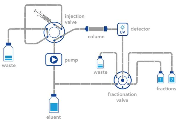
Fig. 1 Flowpath for recycling through pump approach.
