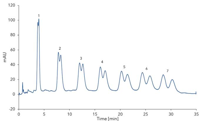
**Fig. 3** Recycling through pump. One measurement with seven cycles (1 to 7); 3.5 mL/min; 100 µL injection of standard with 0.2 mg/mL Rebaudioside A and Stevioside.
