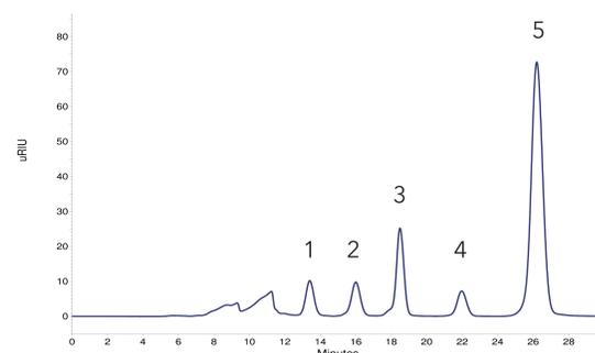
**Fig. 1** Chromatogram of 1:10 dilution of fermentation mash 10  $\mu\text{L}$  injection on Eurokat Ca - 1 xylose (8.2 mg/mL), 2 arabinose (8.3 mg/mL), 3 glycerol (21.0 mg/mL), 4 mannitol (7.0 mg/mL), 5 xylitol (80.6 mg/mL)
