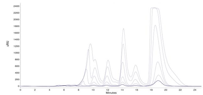
**Fig. A2** Overload studies with semi-preparative Eurokat Ca and fermentation mash; 50  $\mu\text{L}$ , 100  $\mu\text{L}$ , 200  $\mu\text{L}$ , 500  $\mu\text{L}$ , 1000  $\mu\text{L}$ , 1500  $\mu\text{L}$  injection
