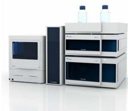
The analysis of saccharides requires an isocratic HPLC system equipped with degasser, autosampler, column oven and a refractive index detector. Other configurations are also available. Please contact KNAUER to configure a system that fits your needs.
