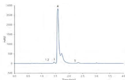
**Fig. A2** Chromatogram of vanilla baking aroma, 1) 4-hydroxybenzoic acid, 2) vanillic acid, 3) 4-hydroxybenzaldehyde, 4) vanillin, 5) coumarin
