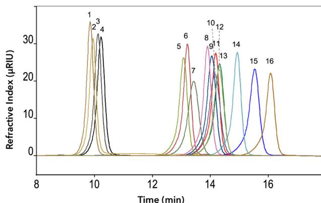
**Fig. 2** Measurement of sugar standards on the Eurokat Na column. Flow rate 0.5 ml/min, temperature 75 °C, sample concentration 2 mg/ml, injection volume 20  $\mu\text{l}$ . Components are listed in **Tab. 3**
