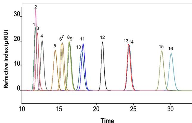
**Fig. 1** Measurement of sugar standards on the Eurokat Ca column. Flow rate 0.5 ml/min, temperature 75 °C, sample concentration 2 mg/ml, injection volume 20  $\mu\text{l}$ . Components are listed in **Tab. 2**
