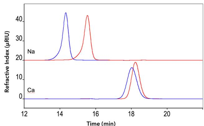
**Fig. 6** Arabinose (red) and fructose (blue) measured with Eurokat Na (above) and Eurokat Ca (below) columns. Flow rate 0.5 ml/min, temperature 75 °C, sample concentration 2 mg/ml, injection volume 20 µl
