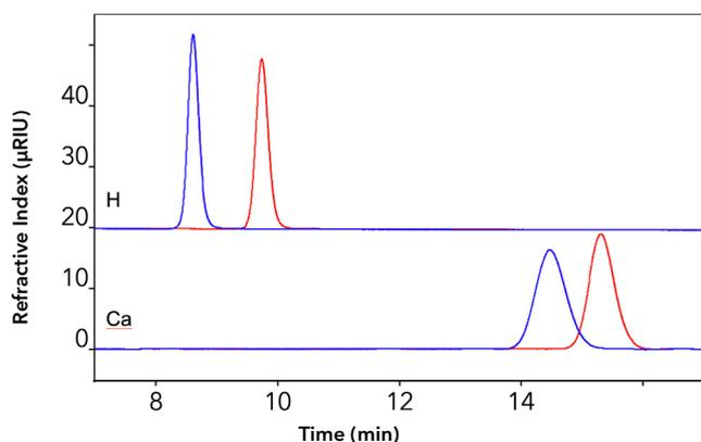
**Fig. 8** Rhamnose (red) and glucose (blue) measured with Eurokat H (above) and Eurokat Ca (below) columns. Ca: flow rate 0.5 ml/min, temperature 75 °C; H: flow rate 0.7 ml/min, temperature 60 °C; sample concentration 2 mg/ml, injection volume 20 µl.
