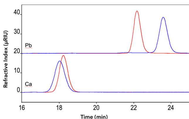
**Fig. 7** Arabinose (red) and fructose (blue) measured with Eurokat Pb (above) and Eurokat Ca (below) columns. Flow rate 0.5 ml/min, temperature 75 °C, sample concentration 2 mg/ml, injection volume 20 µl.
