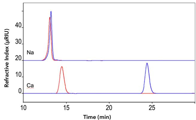
**Fig. 5** Glucose (red) and mannitol (blue) measured with Eurokat Na (above) and Eurokat Ca (below) columns. Flow rate 0.5 ml/min, temperature 75 °C, sample concentration 2 mg/ml, injection volume 20 µl.
