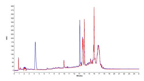
Fig. 2 Overlay of sample (red) and spiked sample (blue) of flexible foam
