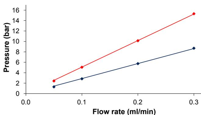
**Fig. 2** Systemic pressure versus flow rate of the AZURA compact system (blue) pressure with capillary connections as described in Figure 1; red with additional 0.13 mm ID tubing to fraction collector
