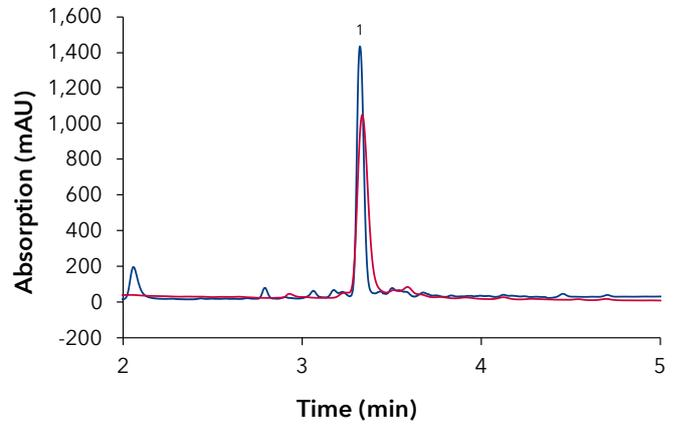
Fig. 2 Particle size comparison; blue: 5 µm; red: 10 µm
