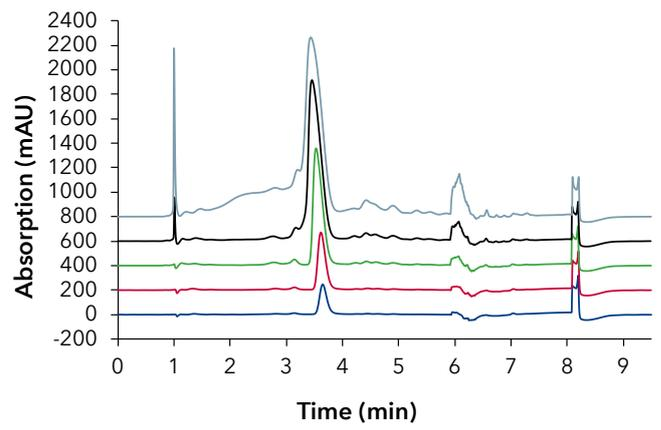
Fig. 4 Top to bottom: 100, 50, 25, 10, 5 µl injection volume
