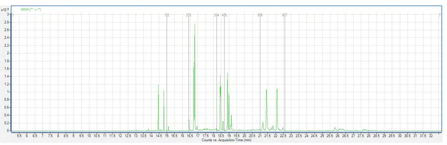
Fig. 2 GC-MS/MS chromatogram of purified soil sample: determination of PAHs
