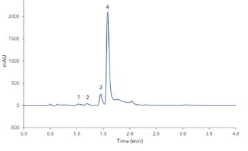
Fig.2 Chromatogram of extracted vanilla bean, 1) 4-hydroxybenzoic acid, 2) vanillic acid, 3) 4-hydroxybenzaldehyde, 4) vanillin
