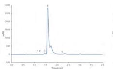
Fig.A2 Chromatogram of vanilla baking aroma, 1) 4-hydroxybenzoic acid, 2) vanillic acid, 3) 4-hydroxybenzaldehyde, 4) vanillin, 5) coumarin
