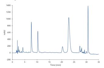
Fig.1 Analytical chromatogram of the crude green tea extract at 220 nm; step gradient separation 10 % acetonitrile until 26 min, then 15 % acetonitrile
