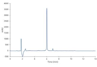
Fig.4 Analytical chromatogram of the third fraction containing epigallocatechin gallate (m/z 457.4; [M-H]<sup>-</sup>); linear gradient separation 5 %-50 % acetonitrile
