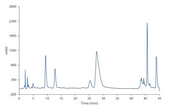
Fig.2 UV chromatogram of a purification run for the crude green tea extract at 220 nm
