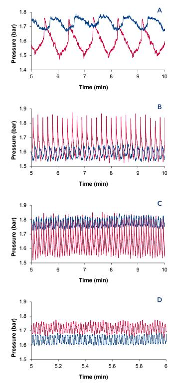
Fig. 2 Overlay of the external pressure signal at different flowrates, approx. 1.5 bar back pressure and water as eluent. Pressure signal without pulse damper (red), pressure signal with pulse damper (blue); (A) 0.1 ml/min; (B) 0.5 ml/min; (C) 1ml/min; (D) 5 ml/min
