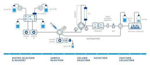
Fig. 1 Example of a typical two step purification system.
