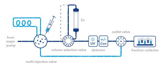
Fig. 4 Flow scheme for the basic set up for two step purification.
