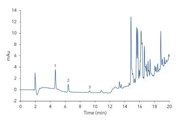
**Fig. 2** Chromatogram of olive oil sample 2. 1 - 3-hydroxytyrosol, 2 - Tyrosol, 3 - vanillic acid.
