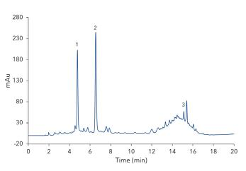
**Fig.5** Chromatogram of olive oil wastewater sample 1. 1 - 3-hydroxytyrosol, 2 - Tyrosol, 3 - Vanillic acid.
