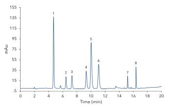
**Fig. 1** Chromatogram of mixed standard at calibration level 5. 1 - 3-hydroxytyrosol, 2 - Tyrosol, 3 - 4-hydroxyphenylacetic acid, 4 - Vanillic acid, 5 - Caffeic acid, 6 - Syringic acid, 7 - Oleuropein, 8 - Quercetin.
