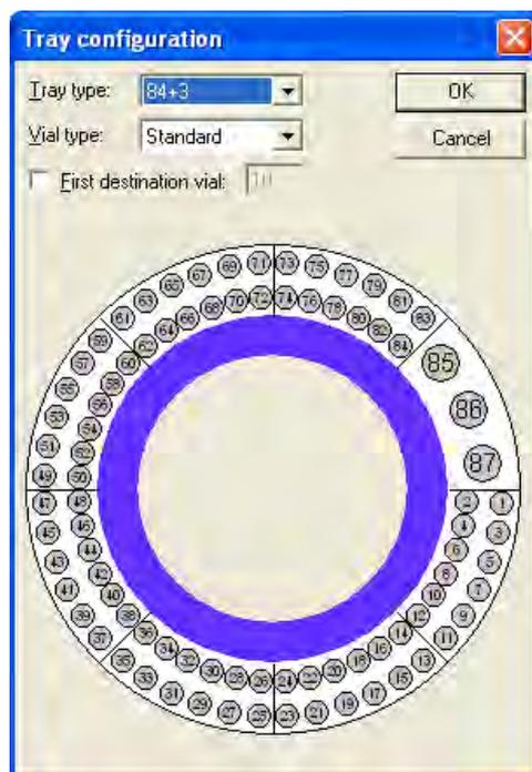
Fig. 97 Tray configuration for the autosampler Knauer Optimas
