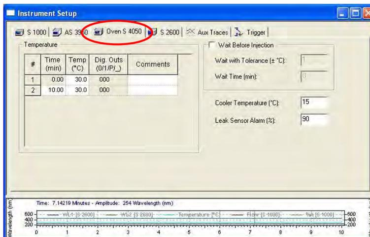
Fig. 192 Setup window, column oven 4050
