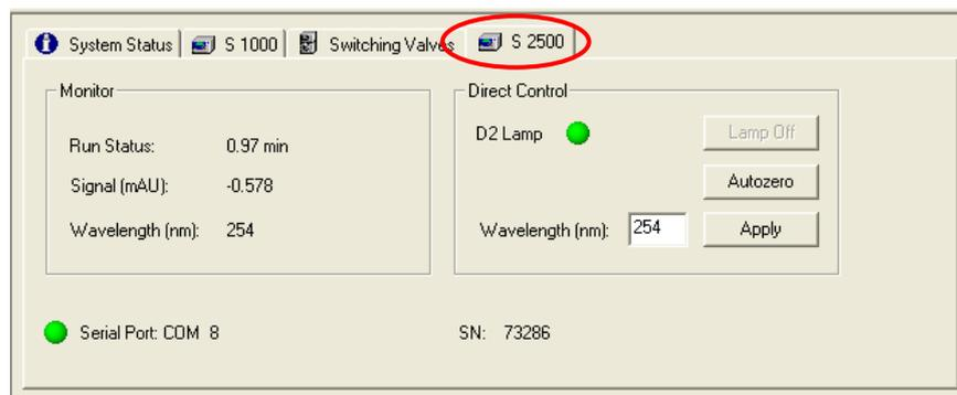
Fig. 218 UV-Detector status tab, example: S 2500
