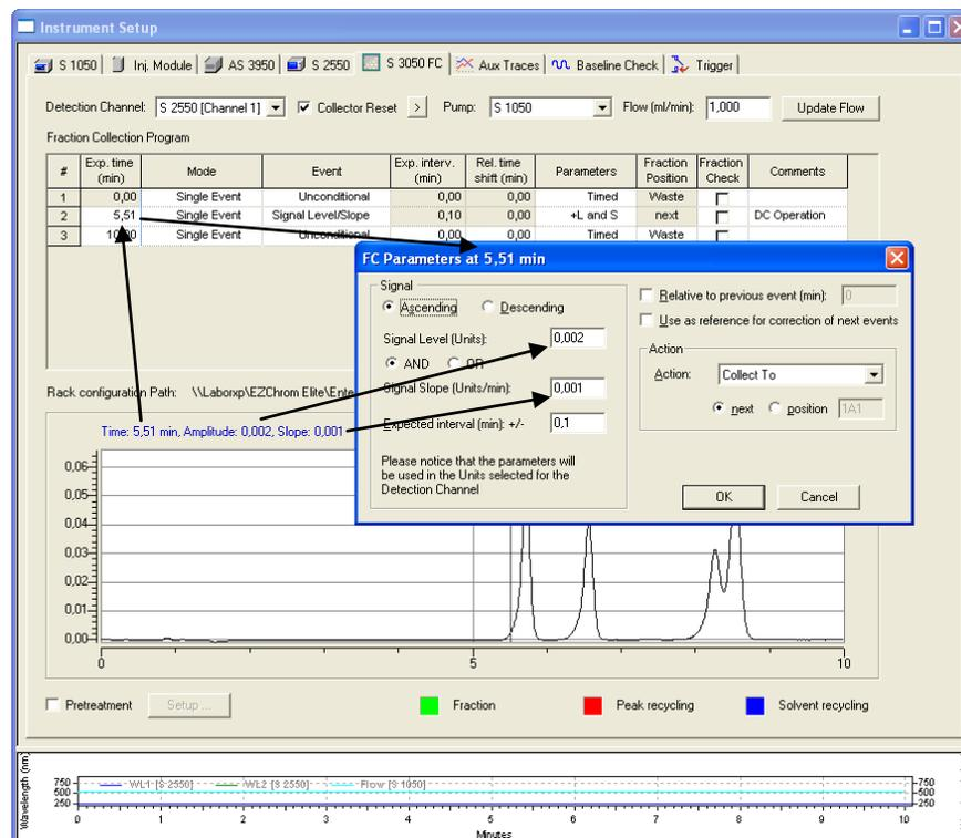
Fig. 351 Programming the fraction table
