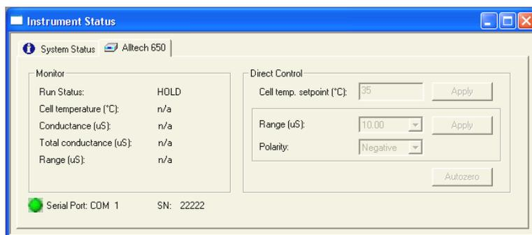
Fig. 228 Detector Status tab, Conductivity Detector Alltech 650
