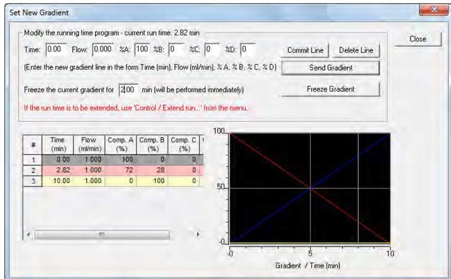
Fig. 212 Gradient modify window – freeze gradient for 2 minutes entered
