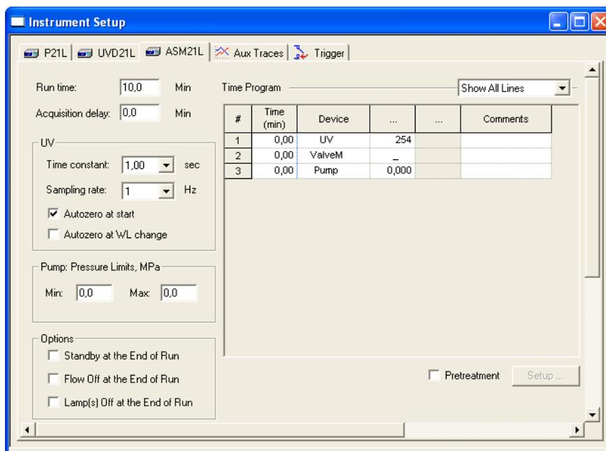
Fig. 160 ASM 2.1L setup window for pump, valve, detector
