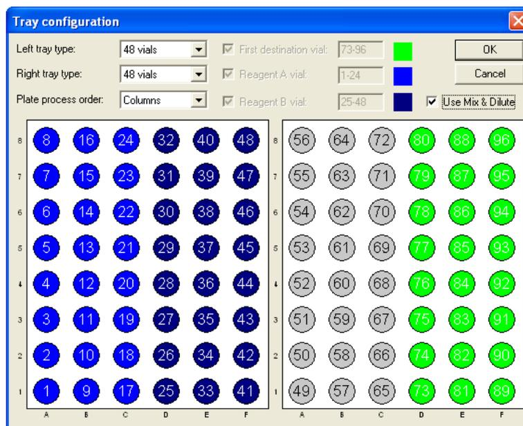
Fig. 95 Tray configuration for the autosampler 3950 with option Use Mix & Dilute
