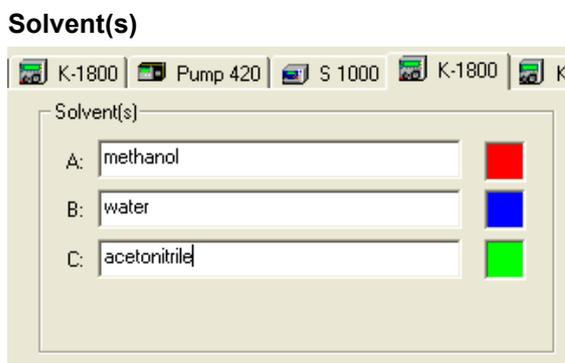
Fig. 125 Solvent description in pump setup window
