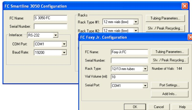
Fig. 320 Fraction collector configuration window
