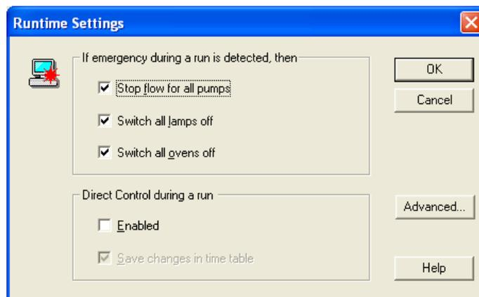
Fig. 249 Knauer Instrument Control Method Option - Runtime Settings
