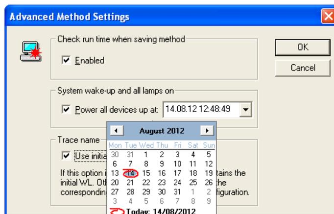
Fig. 252 Advanced Runtime Settings – System wake-up... - date setting
