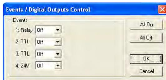
Fig. 137 Configuring Digital Outputs
