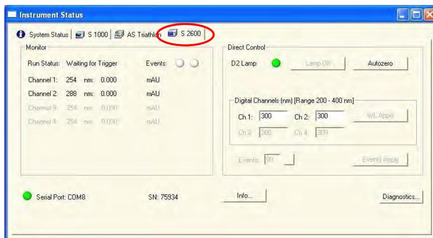
Fig. 223 DAD-Detector status tab, example: DAD 2600
