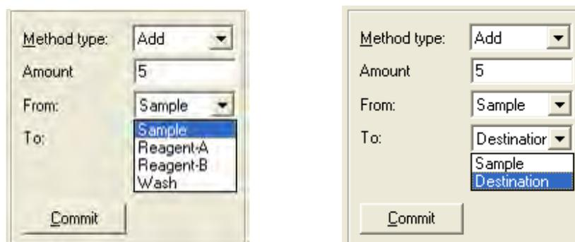
Fig. 166 Autosampler 3900/3950 Mix Step Add
