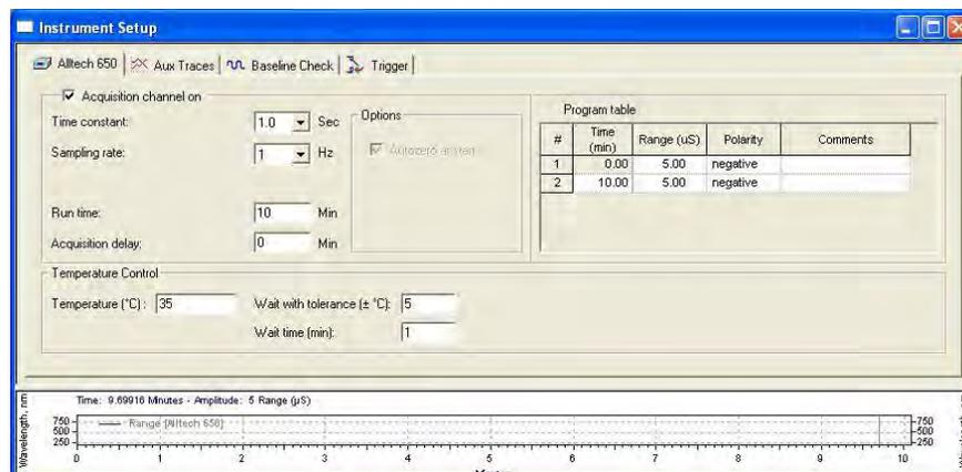
Fig. 154 Alltech 650 conductivity detector setup window
