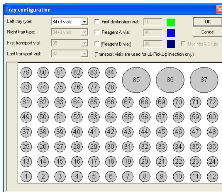
Fig. 94 Tray configuration 84+3 vials for the autosampler 3950
