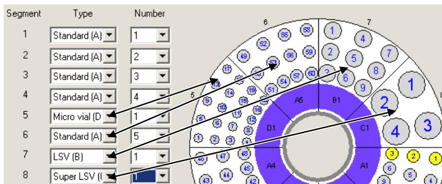
Fig. 103 Tray configuration, displaying different tray types
