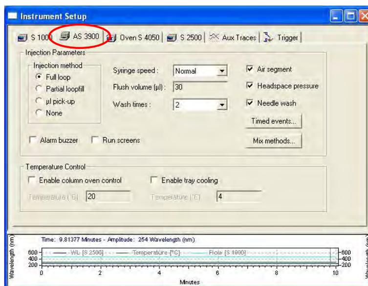
Fig. 163 Autosampler 3900 setup window
