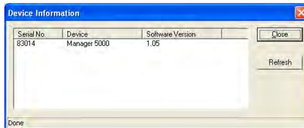
Fig. 230 Device information for connected Manager 5000 interface module
