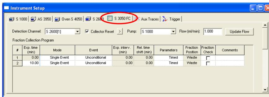
Fig. 328 Fraction collector setup window (upper part)
