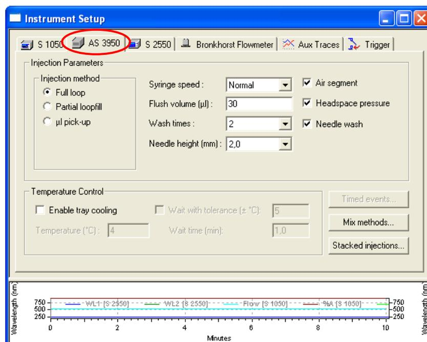
Fig. 169 Autosampler 3950 setup window
