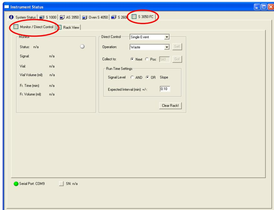
Fig. 353 Fraction Collector status tab - Monitor / Direct control
