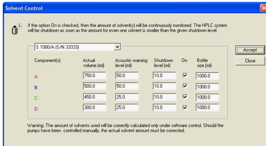
Fig. 257 Solvent Control dialog box (quaternary LPG)
