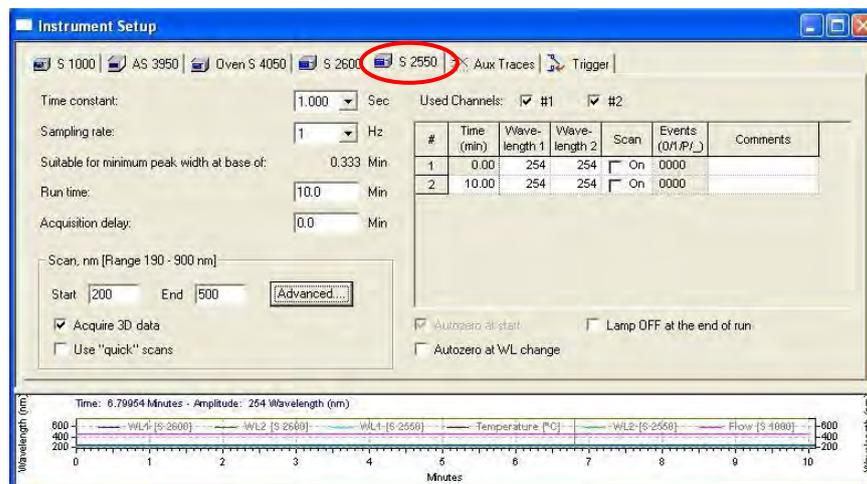
Fig. 143 Detector S 2550 setup window
