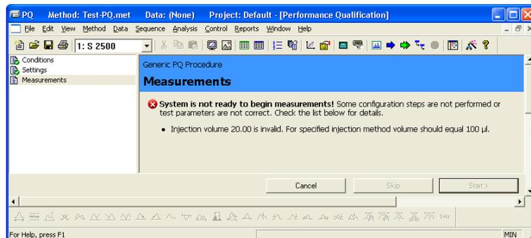
Fig. 263 PQ consistence check, failed
