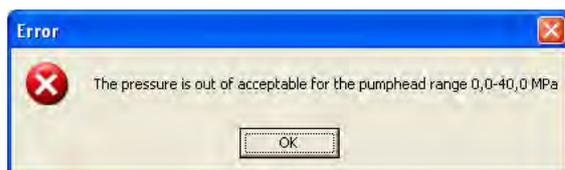
Fig. 124 Error message when pressure limits are out of range
