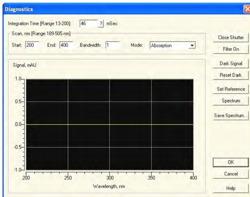
Fig. 225 Diagnostics window of Diode Array Detectors
