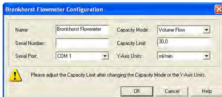
Fig. 117 Configuration window for the Bronkhorst flowmeter
