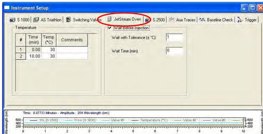
Fig. 193 Setup window, column oven Jetstream
