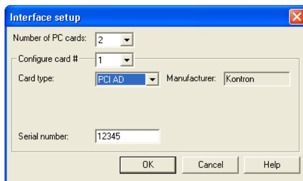
Fig. 34 Dialog box for configuring the Kontron interface card PCI AD
