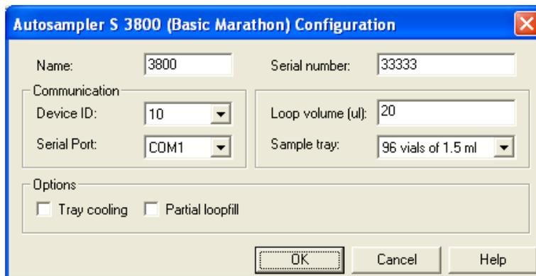
Fig. 98 Configuration window for the autosampler 3800
