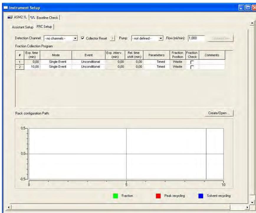
Fig. 161 ASM 2.1L setup window for fractionation valve
