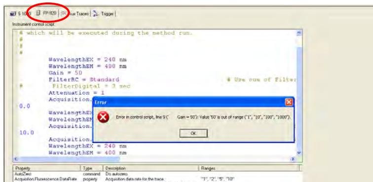
Fig. 276 Instrument setup programming window, example Jasco FP-920
