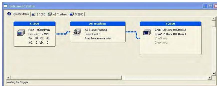
Fig. 29 Instrument Status window, system status tab of a running method
