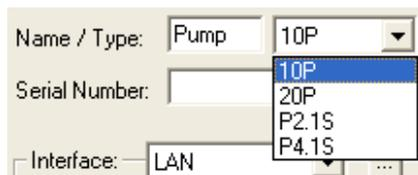
Fig. 49 selection option for pumps 10P, 20P, P2.1S and P4.1S
