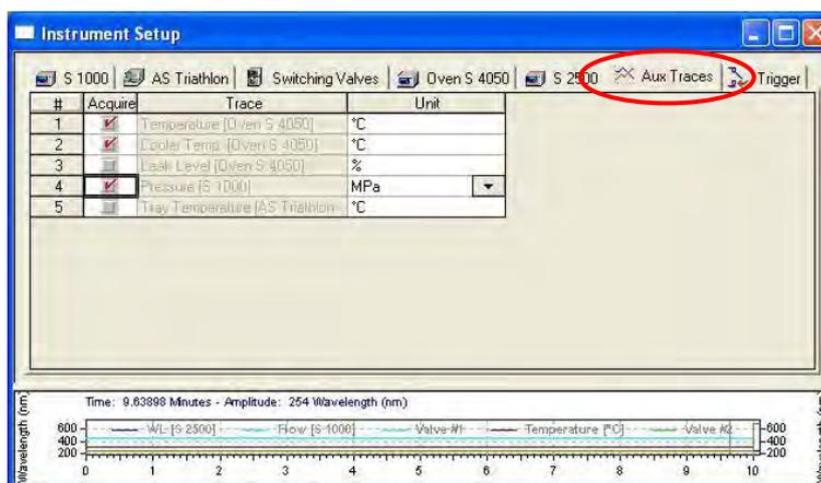
Fig. 195 Setup window, Auxiliary Traces Any configured HPLC system with at least one pump with pressure transducer, a column oven or a flowmeter will be completed by an additional tab for auxiliary traces.
