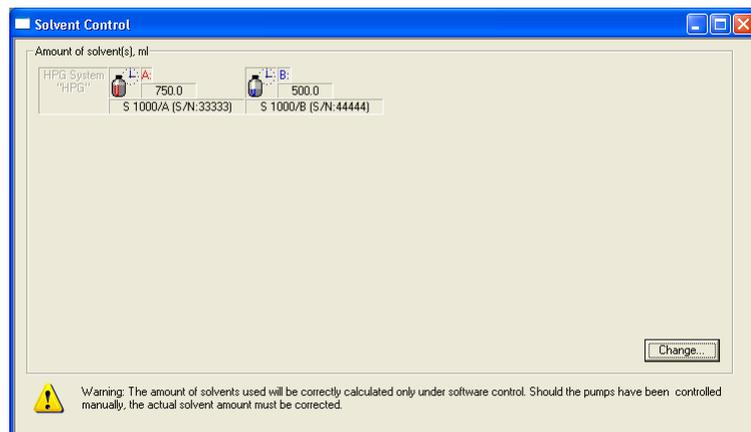
Fig. 258 Solvent Control window – binary HPG system
