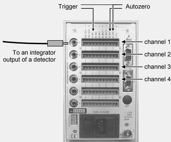
Fig. 82 Cable connections to the Knauer Interface Box, Model 96
