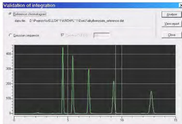
Fig. 267 Validation of Integration dialog window, real chromatogram
