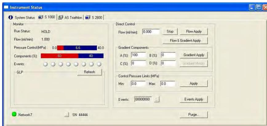
Fig. 202 Instrument status tab, example: Smartline Pump 1000
