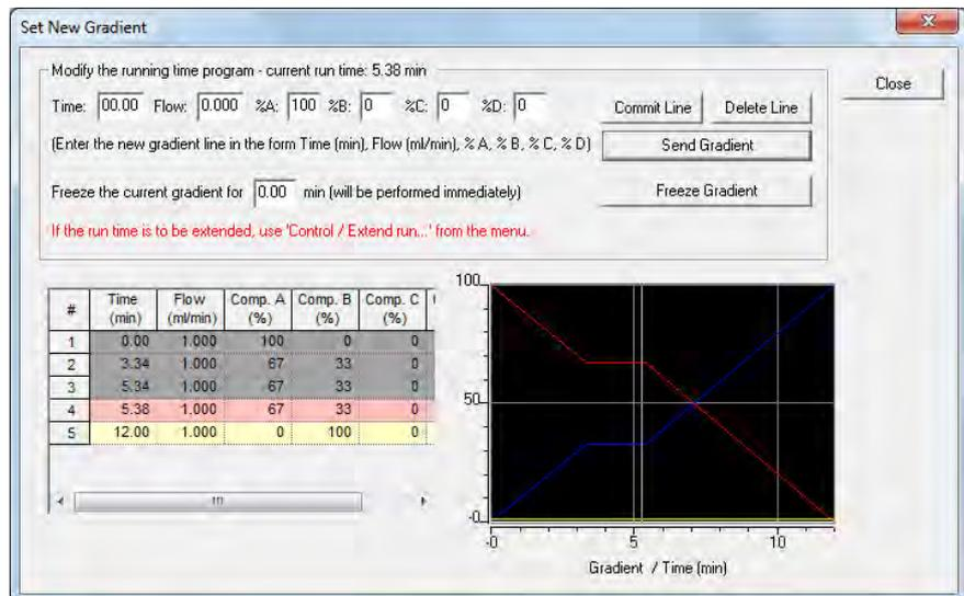
Fig. 213 Gradient modify window – freeze gradient for 2 minutes executed
