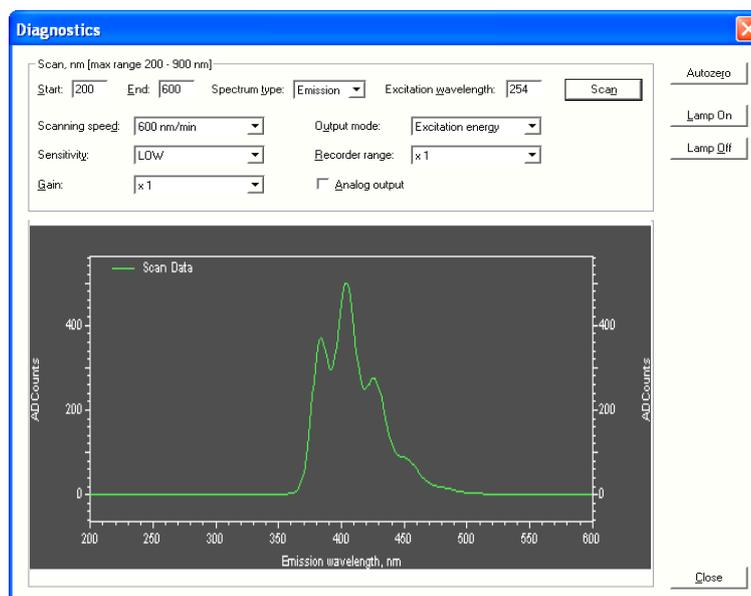
Fig. 227 Diagnostics window of Fluorescence Detector RF-10AxI with an anthracene spectrum
