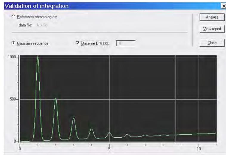
Fig. 269 Validation of Integration with baseline drift
