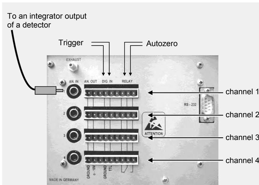
Fig. 83 Cable connections to the Manager 5000/5050 or IF2
