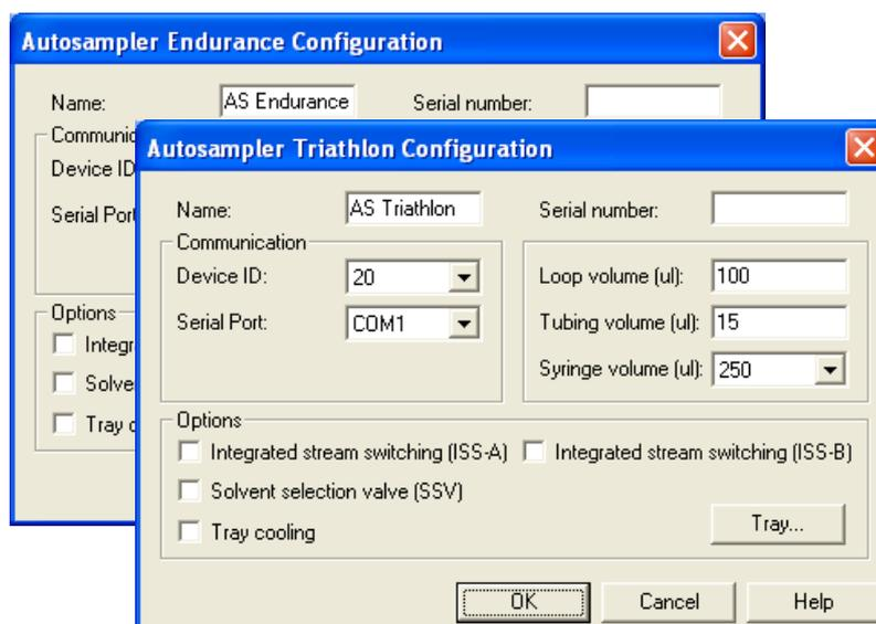
Fig. 101 Configuration windows for the autosamplers Triathlon and Endurance
