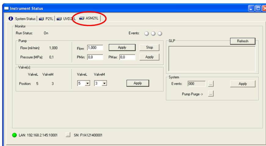
Fig. 232 ASM2.1L status tab – valve, valve, pump
