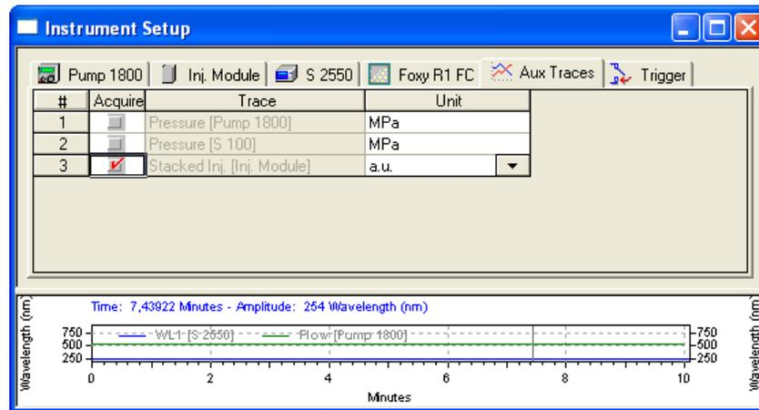
Fig. 364 Injection Module Stacked injections auxiliary trace
