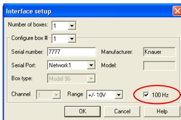
**Fig. 33** Dialog box for configuring the Model 96 Interface Box with activated 100 Hz option
