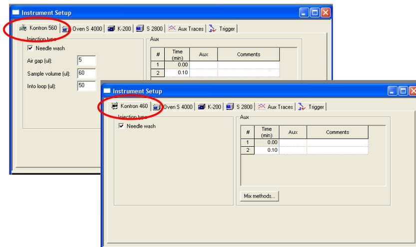
Fig. 182 Kontron Autosamplers setup window
