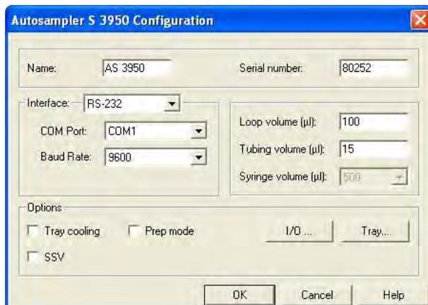
Fig. 90 Configuration window for the autosampler 3950
