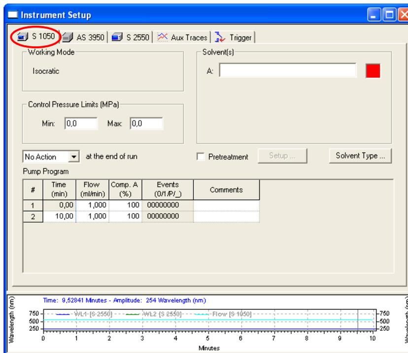
Fig. 120 Instrument setup window (Smartline Pump 1050)
