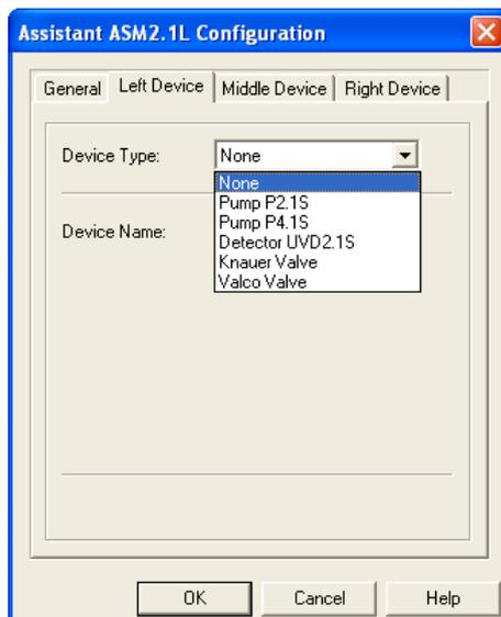
Fig. 89 Configuration windows left device tab, device type selection
