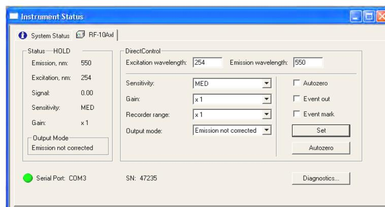
Fig. 226 Detector Status tab, Fluorescence Detector RF-10AxI
