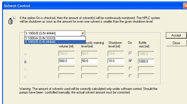
Fig. 259 Solvent Control dialog box – HPG system
