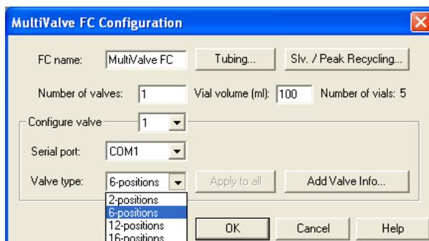
Fig. 325 Multi valve fraction collector configuration window
