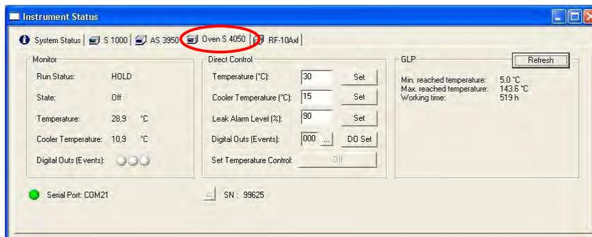
Fig. 246 Status tab, column oven 4050
