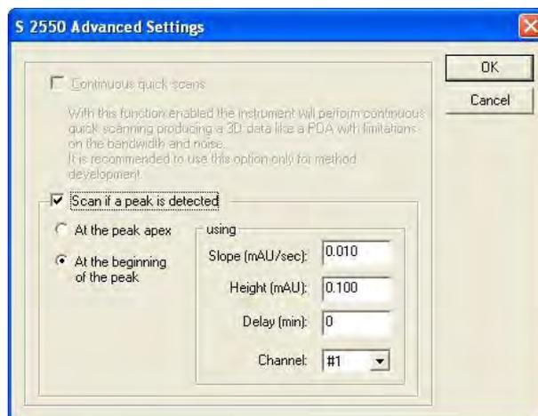
Fig. 145 Detector S 2550 Advanced setup window
