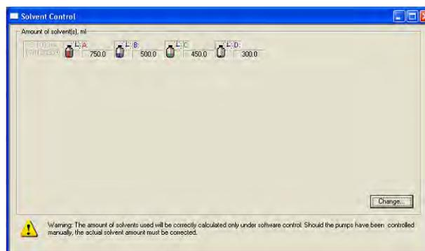
Fig. 256 Solvent Control window (quaternary LPG)
