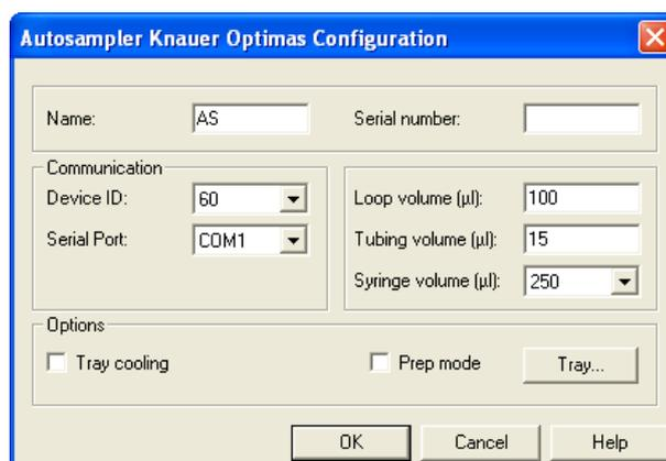
Fig. 96 Configuration window for the autosampler Knauer Optimas
