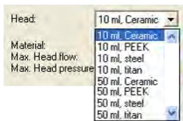
Fig. 54 Available pump heads for K-1001, K-1000, K-501, and K-120 pumps
