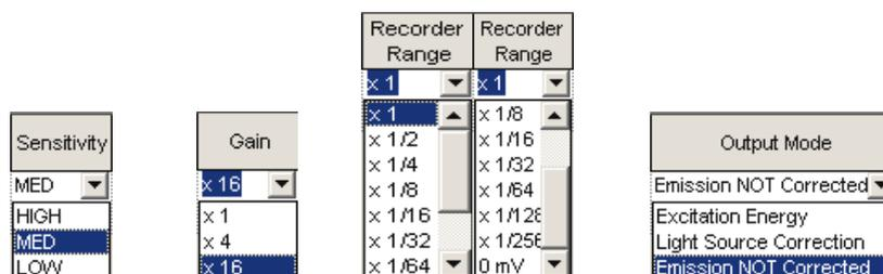
Fig. 153 pull down menus in the Fluorescence Detector RF-10Ax1 setup
