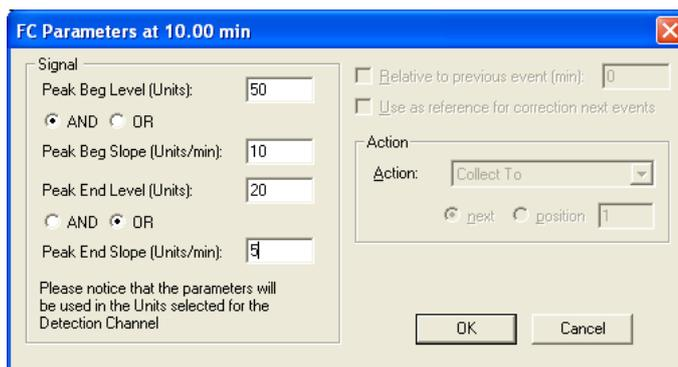
Fig. 337 FC parameters Signal Level/Slope (Peak Recognition)
