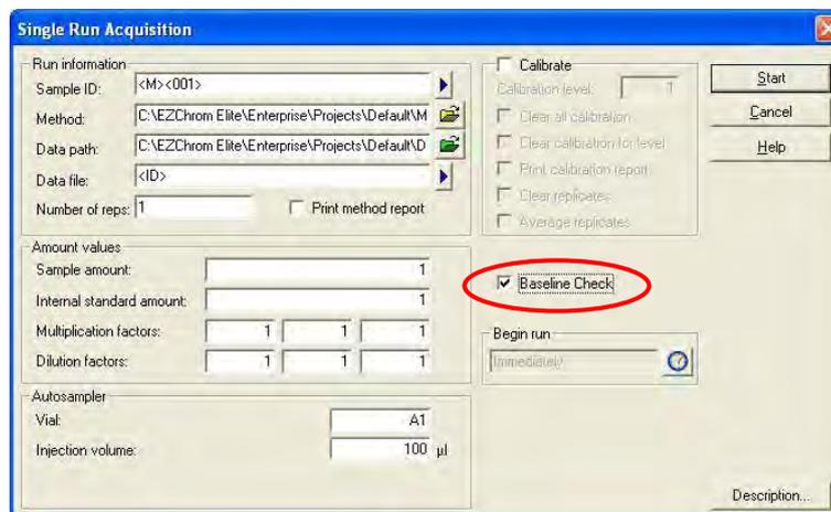
Fig. 199 Activating the baseline check for a single run
