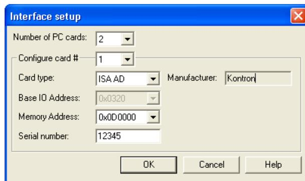
Fig. 35 Dialog box for configuring the Kontron interface card ISA AD
