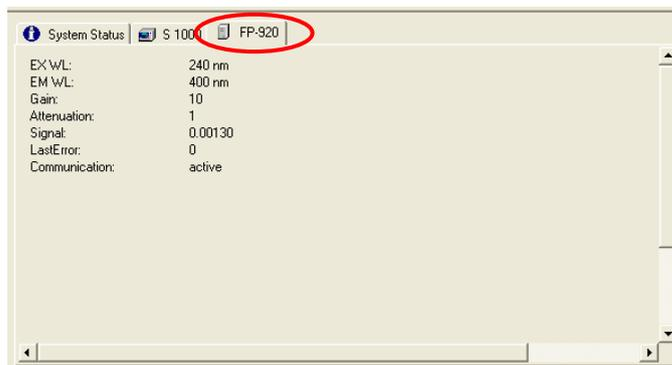
Fig. 277 Instrument status tab, example Jasco FP-920
