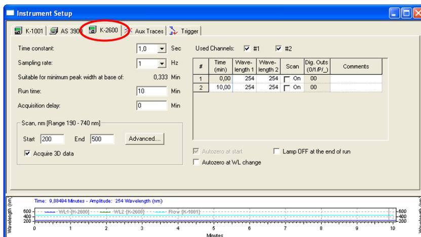
Fig. 139 Detector K-2600 setup window with PDA option
