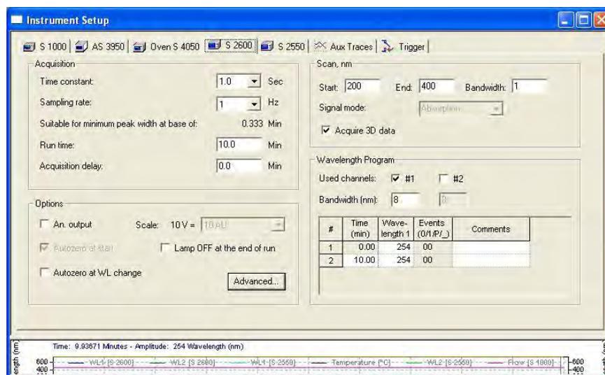
Fig. 147 Detector S 2600 setup window with PDA option
