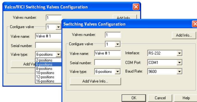
Fig. 109 Configuration window for the Switching Valves
