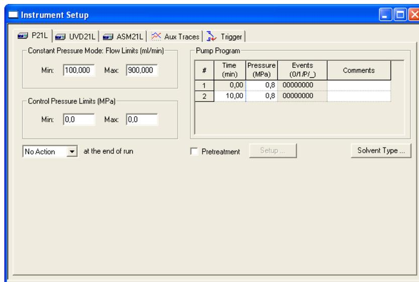
Fig. 132 Instrument setup window P2.1L constant pressure mode (isobar)
