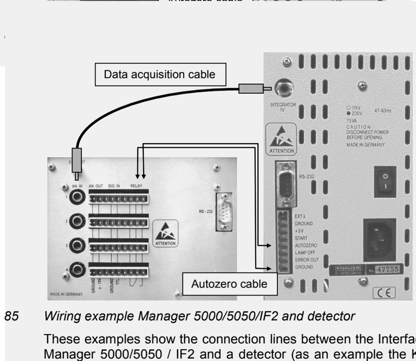
Fig. 85 Wiring example Manager 5000/5050/IF2 and detector
