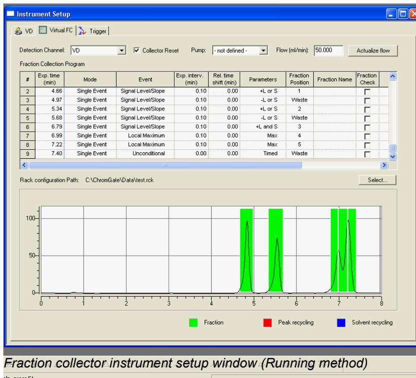
Fig. 356 Fraction collector instrument setup window (Running method)
