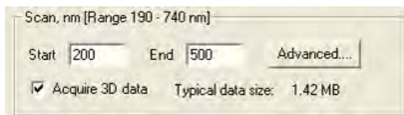
Fig. 140 Detector K-2600 setup window with PDA option
