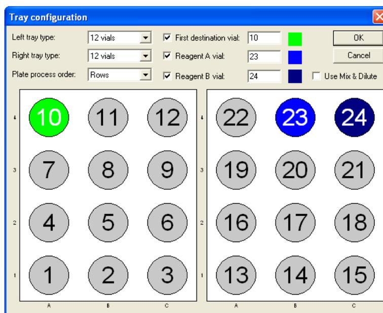
Fig. 93 Tray configuration for the autosampler 3950
