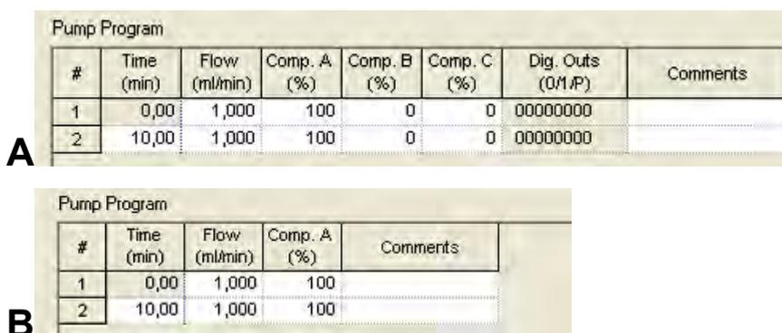
Fig. 129 Pump program in pump setup window: **A** Pump 1800 LPG, **B** K-501 isocratic
