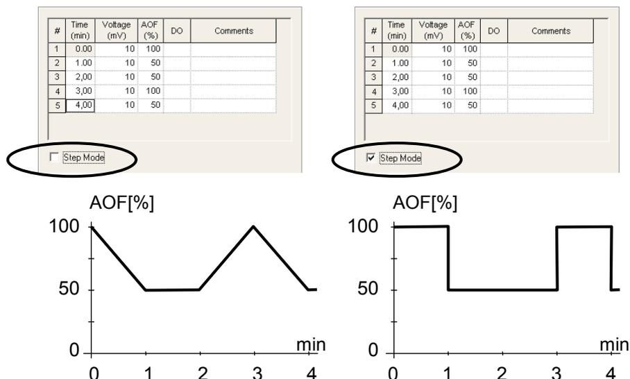
Fig. 188 Analog output profile without and with activated Step Mode
