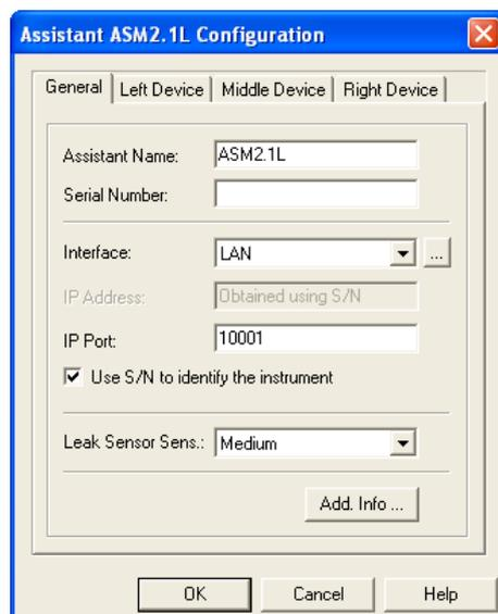
Fig. 86 Assistant ASM2.1L configuration window, tab General
