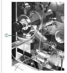
**Fig. 40:** Loosen the screw fitting of the inline filter cartridge
