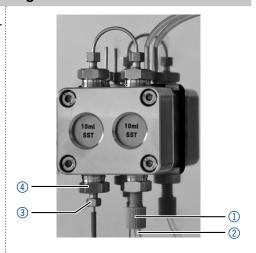
Fig. 33: Removing fittings and tubings
