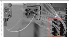
Fig. 14: 4-channel degasser with valve block
