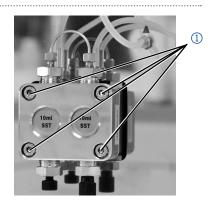
Fig. 35: Removing screws
