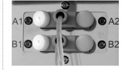
**Fig. 12:** Solvent selection valve with cap fitting
