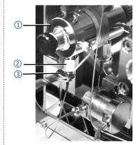
Fig. 39: Loosen the capillary
