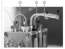
Fig. 17: Connecting piston backflushing
