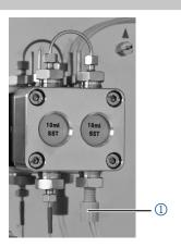
Fig. 10: Solvent line on pump head
