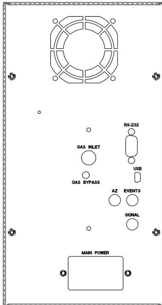
Figure 6. Rear Panel of the detector
