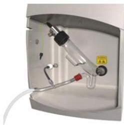
*Figure 32. Disconnecting fluids inlets*
