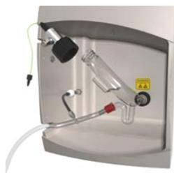
Figure 33. Removing the nebulizer
