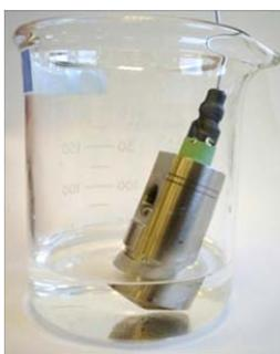
Figure 35. Nebulizer Cleaning (not more than 2 cm of cleaning liquid)
