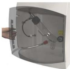
*Figure 31. Front window removal*
