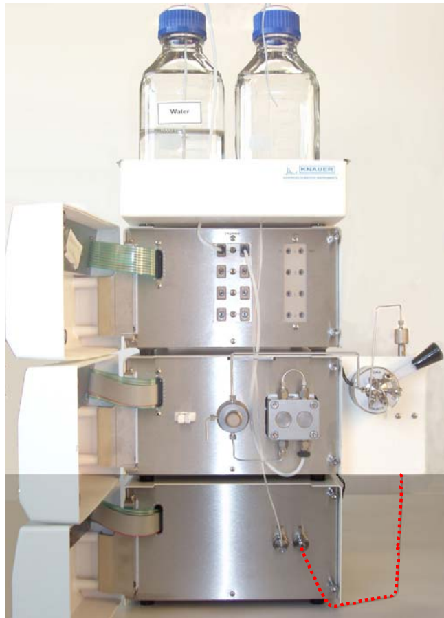
Fig. 11 Capillary Connections of the Detector
