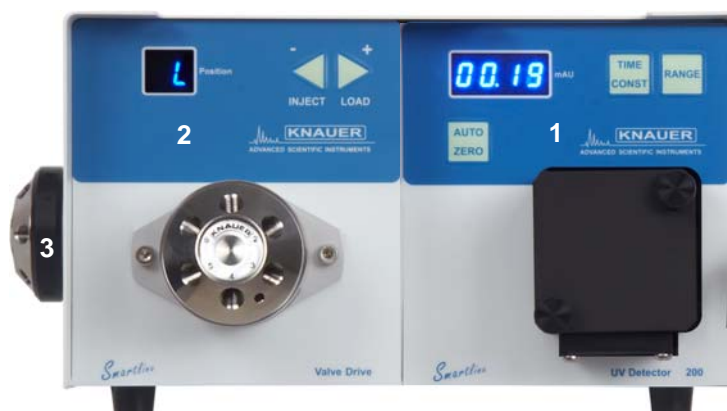
Fig. 7 Front view of the Smartline Assistant 6000 (A5003V416), with: 1 Smartline UV Detector 200 2 6-Port-2-channel injection valve and 3 13-Port-1-channel switching valve for fraction collection
