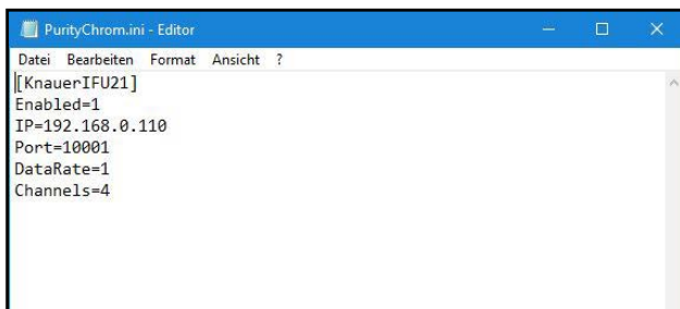
Fig.3 Configuration example for IFU 2.1 LAN
