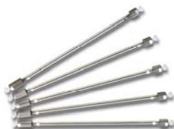
The ProntoSIL C18 ace-EPS belongs to the new group of stationary RP supports with polar embedded groups. The packing is very stable over a wide pH range (pH 1-10). In comparison to a classical bonded C18 column acidic compounds show a higher retention whereas basic compounds show a slight decrease of retention on an embedded polar column.
