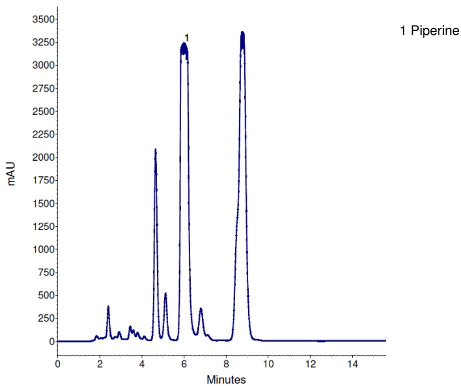
Now the AZURA preparative HPLC system and a Eurospher II C18 phase filled in the KNAUER Vertex Plus AX hardware with axial compression were used. The resulting preparative chromatogram can be seen in fig. 4. The marks indicate when the Piperine fraction was collected to reach the highest purity.
