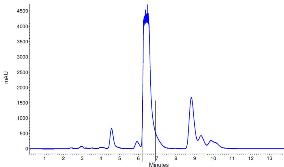
The Piperine fraction was collected using a switching valve. To control the purity of this fraction, the next step was a high resolving HPLC method using the BlueShell classic core shell column and the AZURA compact system. The highest resolution is needed in this step, because all impurities have to be separated from the target peak Piperine to discover the purity of the target substance. The chromatogram of the Piperine fraction's purity control can be seen in figure 5.
