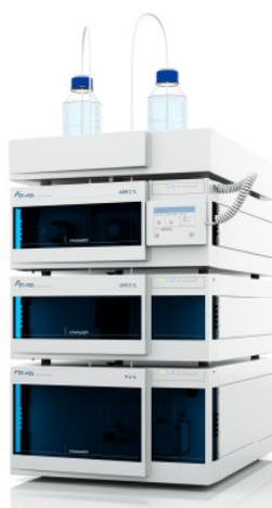
The AZURA Preparative HPLC system is a complete preparative low pressure gradient HPLC system for purification of milligram and gram samples. It consists of a preparative HPLC pump with LPG valve block, a UV/VIS detector and a customizable combination module. The pump P 2.1L with LPG valve block enables to form dynamically eluent mixtures from up to 3 different eluents, or to run a binary gradient.
