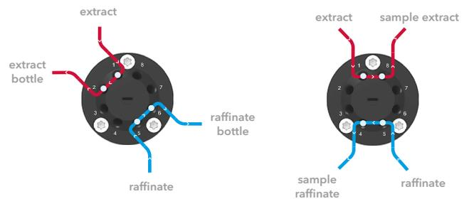
Fig. 3 Operation mode of the sampling valve (8-port 2-position).
