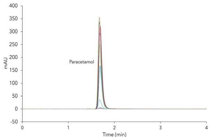
Fig. 4 Increasing concentrations of paracetamol in raffinate during process start-up, samples taken from cycle 1 - 8, 10 and 12. Whole cycles were collected.
