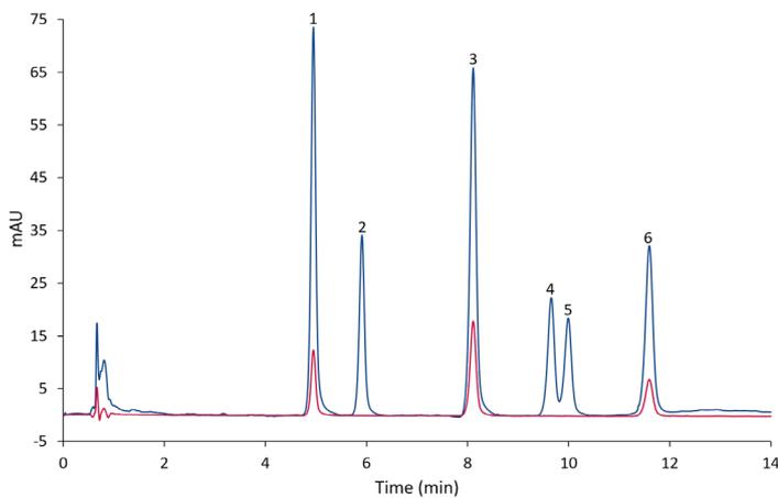
**Fig. 1** Chromatogram of a 10 µg/mL standard mix measured with the DAB method; R=1.3 between  $\Delta^8$ -THC and  $\Delta^9$ -THC; blue - 225 nm, red - 306 nm, 1 - CBDA, 2 - CBD, 3 - CBN, 4 -  $\Delta^9$ -THC, 5 -  $\Delta^8$ -THC, 6 -  $\Delta^9$ -THCA.
