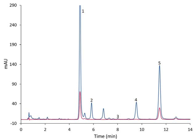
**Fig. 2** Chromatogram of a 1 mg/mL bediol sample in ethanol; blue - 225 nm, red - 306 nm, 1 - CBDA, 2 - CBD, 3 - CBN, 4 -  $\Delta^9$ -THC, 5 -  $\Delta^9$ -THCA.
