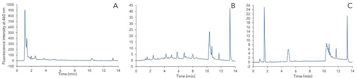
Fig. 2 Three different samples during extraction process. After the extraction with MeOH/H<sub>2</sub>O (A), before SPE (B) and after the SPE extraction (C).
