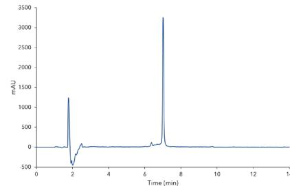
**Fig. A3** Analytical chromatogram of the fourth fraction containing epicatechin gallate ( $m/z$  441.4;  $[M-H]^-$ ); linear gradient separation 5%-50% acetonitrile.
