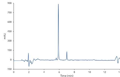
**Fig. A2** Analytical chromatogram of the second fraction containing epicatechin ( $m/z$  289.2;  $[M-H]^-$ ); linear gradient separation 5%-50% acetonitrile.
