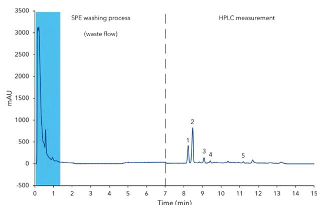
**Fig. 1** Measurement of washing process; blue area: matrix; 1) rebaudioside A, 2) stevioside, 3) rebaudioside C, 4) dulcoside A, 5) steviolbioside; 20  $\mu$ L injection of Stevia extract; 0-7 min) measuring of SPE Washing Process, 7-15 min) measuring of HPLC
