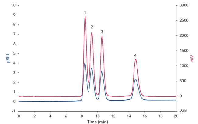
**Fig. 1** ELSD trace (red) and RID trace (blue) of a mixed standard at 0.60 mg/mL; 1) sucrose, 2) maltose, 3) glucose, 4) fructose
