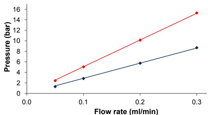
**Fig. 2** Systemic pressure versus flow rate of the AZURA compact system (blue) pressure with capillary connections as described in Figure 1; red with additional 0.13 mm ID tubing to fraction collector
