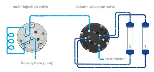
Fig. 3 Connection of the column selection valve.
