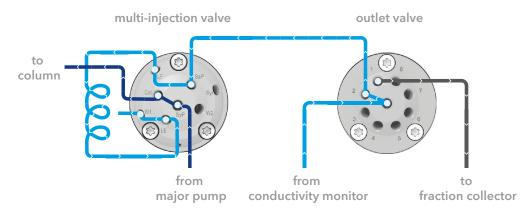
Fig. 4 Connection of the outlet valve.
