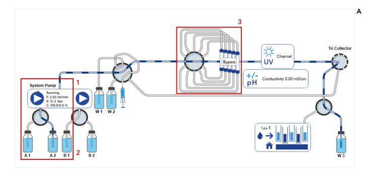
the UV detector and the multiinjection valve for "Peak storage stop". At the end of the run purified protein is stored in the injection loop and can be further purified via the second column in the next step without manual interference.
