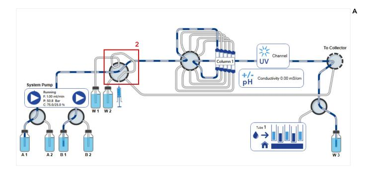
After the sample injection and an isocratic washing step, the elution starts after 5 ml with beginning of the gradient (**Fig. 6 B.1**). At this time point the multi-injection valve should be switched back to the manual load position (**Fig. 6 A+B.2**).
