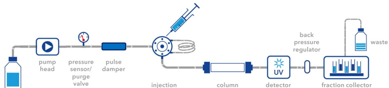
Fig. 3 Flow scheme of AZURA SEC FPLC System with pulse damper behind the pressure sensor
