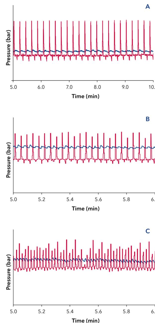
**Fig. 2** Overlay of the external pressure signal at different flowrates, approx. 1.5 bar back pressure and water as eluent. Pressure signal without pulse damper (red), pressure signal with pulse damper (blue); (A) 0.1 ml/min; (B) 0.5 ml/min; (C) 1ml/min
