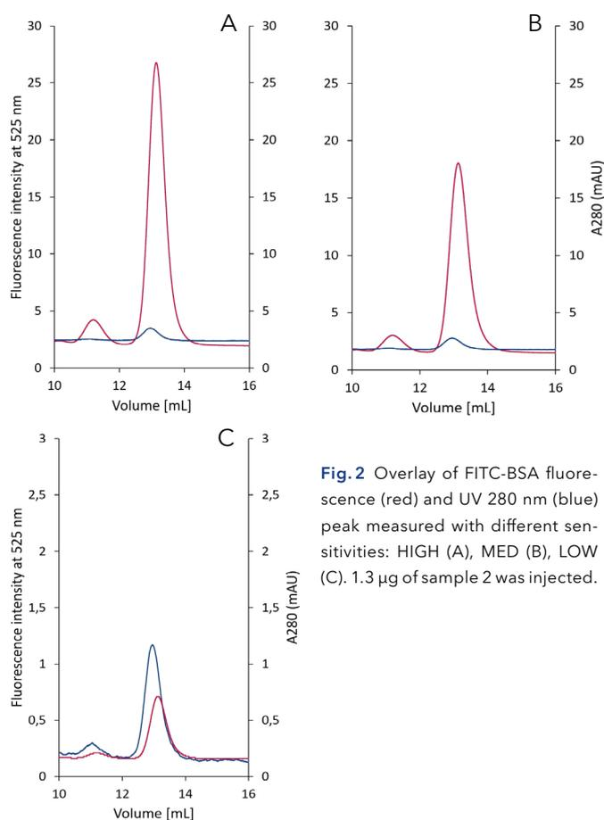
**Fig. 2** Overlay of FITC-BSA fluorescence (red) and UV 280 nm (blue) peak measured with different sensitivities: HIGH (A), MED (B), LOW (C). 1.3  $\mu\text{g}$  of sample 2 was injected.
