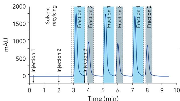
Fig. 2 Chromatogram of three stacked injections; 500  $\mu$ L injection volume per injection; flowrate 25 mL/min; eluent 25/75 ethanol/water (v/v); ambient temperature; automated fractionation.
