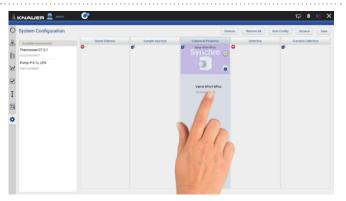
**Fig. 5-21** Drag and drop of the second valve
