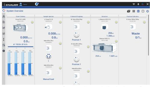
Fig. 5-39 System Overview of a pump showing the level indicator of Eluent Control
