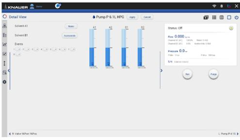
Fig. 5-38 Detail View of a pump showing the level indicator of Eluent Control
