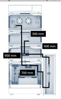
System 4: AZURA® analytical with manual injection, DAD and RI detector
